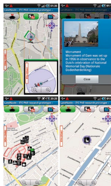
Figure 3: Actual appearance of the interface, with examples of the technical solutions (dual map, a pop-up window with a selected-angle landmark photo, multi-paths, and landmark visibility indication)
