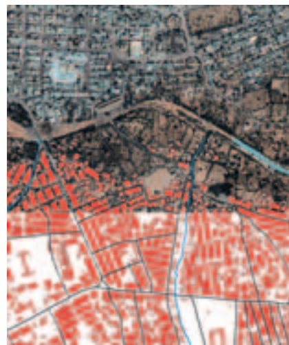
Properties (building blocks and stand-alone properties are indicated) created through on-screen digitising of a Quickbird image and field verification
